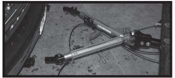
**Step 4.** Position the vehicle to be towed approx.24" behind the towing vehicle. Perform a tow bar safety check, look for any loose fasteners, condition of safety cables, excessive movement in connecting leg shaft when the shaft is extended and locked. If any excessive movement or loose fasteners, the tow bar will need to be serviced before towing. The vehicles **do not** have to be in straight alignment to complete the hook-up. **Engage towed vehicle and towing vehicle parking brake.**
