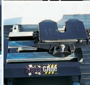
*Cab to trailer interference would normally be an issue on a shortbed, fifth-wheel combo, but the SuperGlide slides back up to 14 inches when the truck turns a corner to provide the necessary clearance. The SuperGlide also includes a base plate that bolts onto the trailer’s pin box.*
