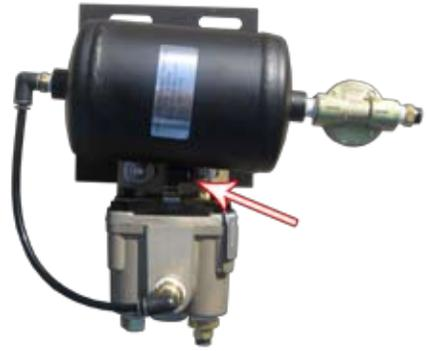
2. Connect the towed-vehicle air hose (from Step 4) to the pushlock connector on the relay valve labeled “DEL.”
