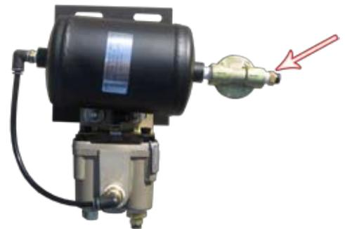
Note: Should you find it necessary to remove an air hose, push the air hose in with one hand, push on the outside ring of the pushlock connector with the other hand, and then pull the air hose out. The ring will release the air hose.
