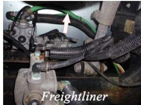
1. Locate the coach's supply air hose. This line goes from the service relay valve to the rear air tank. It is 5/8" in outside diameter. Although it is normally green, it may be any color. Do not confuse this hose with the treadle-valve hose. This line is only 3/8" in outside diameter and should not be tampered with.
