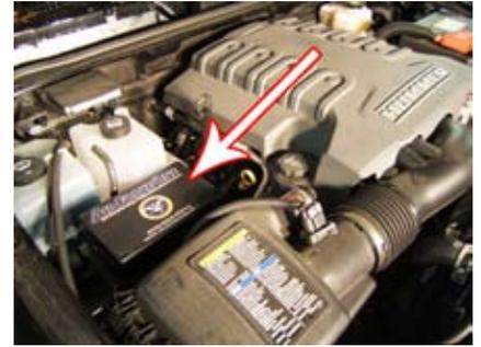
2. Secure the box with either screws or wire ties through the mounting flanges on the box.
